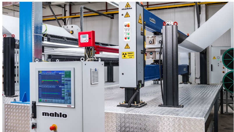
Control of basis weight and moisture on a Spunlace-Nonwoven system (courtesy of Selcuk Iplik Sanayi ve Ticaret A.S.)
