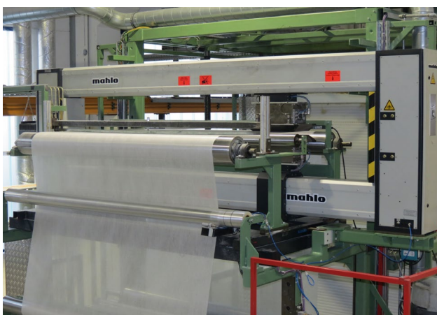
Checking the basis weight with the Gravimat DFI beta sensor in the O-frame Webpro M for the production of screen reinforcements from fibreglass and nonwovens.
