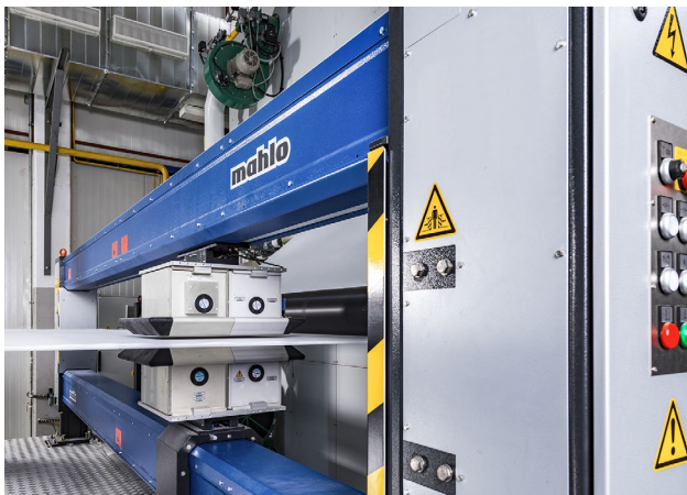
A Qualiscan QMS with a Webpro M scanner measures basis weight with beta sensor and moisture with an infrared sensor.
