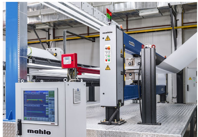
The traversing scanner of the Qualiscan QMS allows generating precise lateral and longitudinal profiles of parameters such as basis weight, thickness or moisture. They are presented clearly arranged in the operating software of the Mahlo system on a touchscreen (in the foreground).
