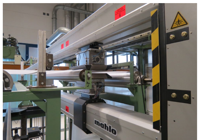
The beta sensor measures basis weight via isotope rays. Complete insensitivity to web flutter across the entire measuring gap through DFI technology (Dynamic Flutter Independent). Even smallest beta ray sources thereby achieve their maximum measuring performance.
