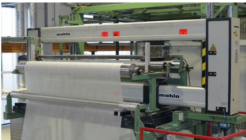
Basis weight control with the production of screen reinforcements from glass fibres and nonwovens (courtesy of Kirson Industrial Reinforcements GmbH)
