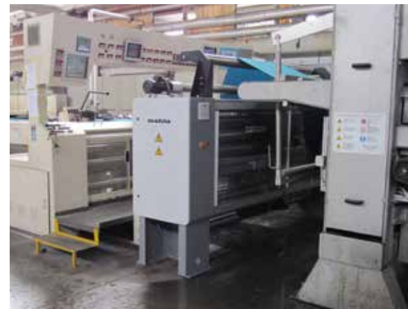
Classic feed-end straightener in textile production
