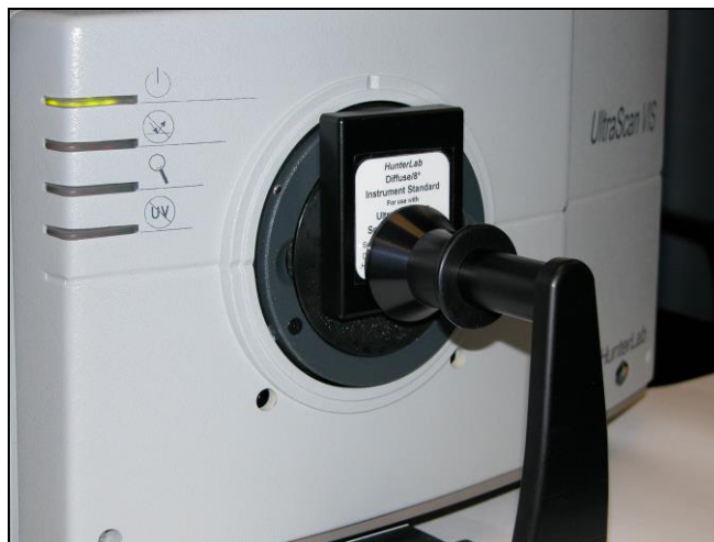
Figure 25. Standardizing on the White Tile
