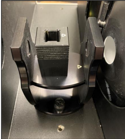
Figure 88. Cell Holder Installed
