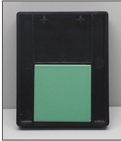
Figure 47. Green Tile at Reflectance Port
