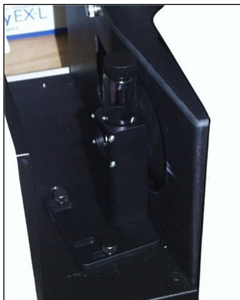
Figure 76. Tube Holder Installed
