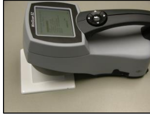
Figure 66. Using a White Tile Backing
