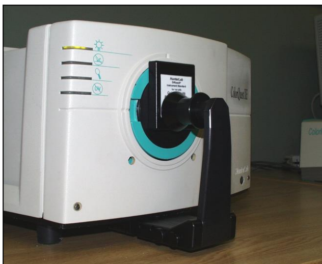
Figure 15. Setting Top-of-Scale with the White Tile
