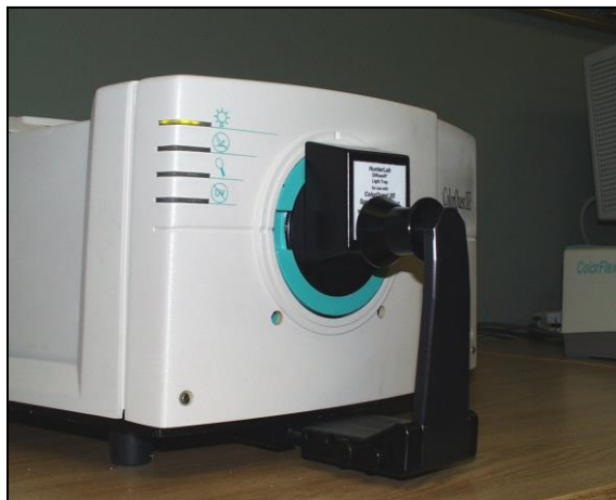
Figure 12. Standardizing on the Light Trap to set Bottom-of-Scale
