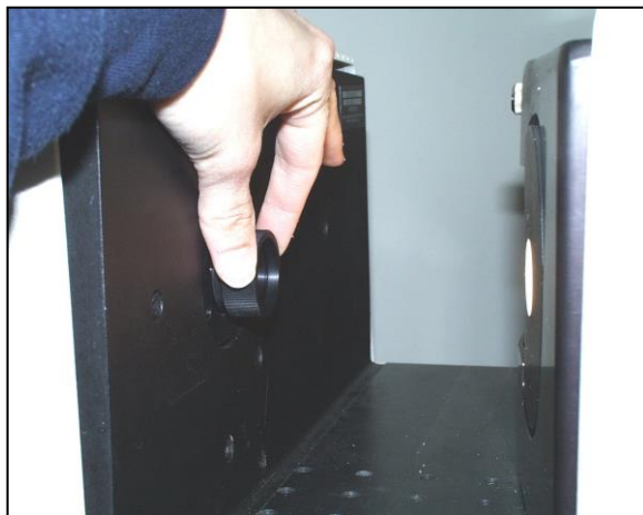
Figure 237. Inserting the Didymium Filter at RTRAN port (lens side)
