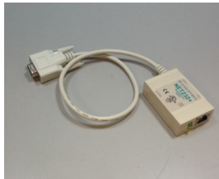
Figure 18. Ethernet to RS-232 Converter for Connection via Serial Port
