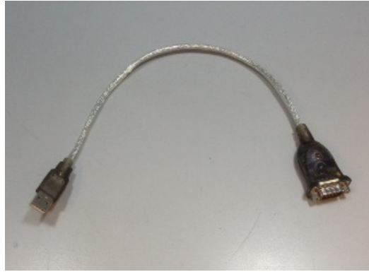
Figure 19. RS-232 to USB Converter for Connection via USB Port
