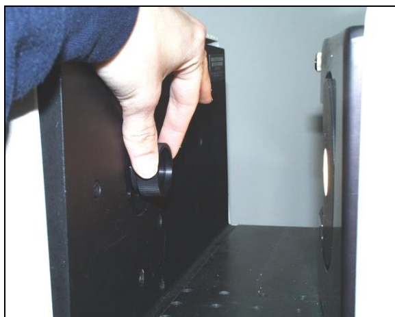
Figure 42. Didymium Filter Test: Place filter at RTRAN port
