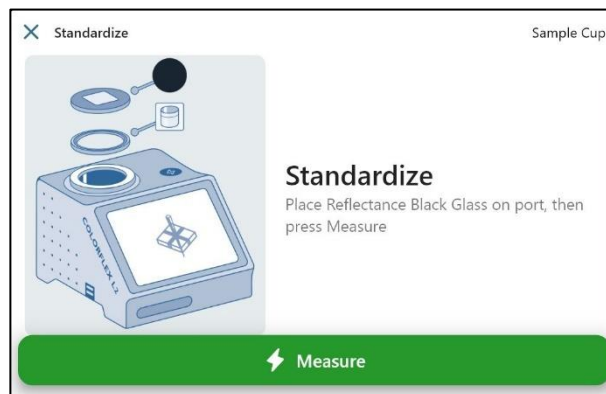
Figure 5. Measure Reflectance Black Glass
