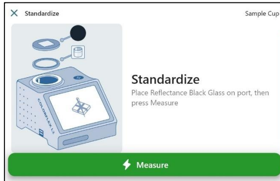
Figure 2. Measure Reflectance Black Glass
