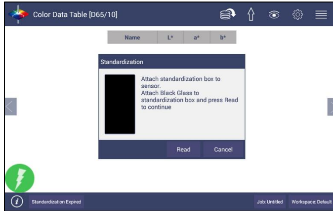
Figure 6. Read the Black Glass for Bottom-of-Scale
