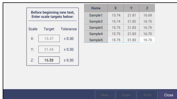
Figure 80. Green Tile Readings
