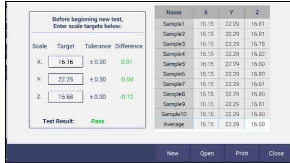
Figure 11. Green Tile Readings
