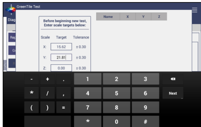
Figure 10. Input Target Values for Green Tile
